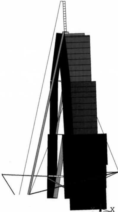
**Figure 15** Tension and compression forces in the rig, FEA, AWA 135
