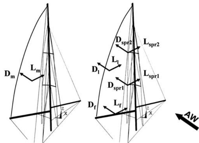
Figure 4 Applying drag and lift forces from the main on the rig
