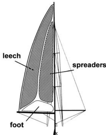
**Figure 5** Sizes of areas from the mainsail corresponding with parts of the mainsail force
