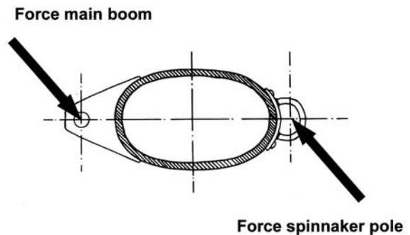
**Figure 17** Initiating torque in mast panel 1
