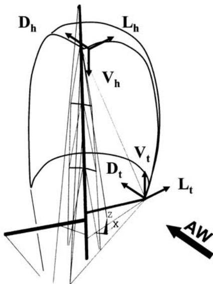
Fig. 9 Applying forces of the spinnaker on the rig
