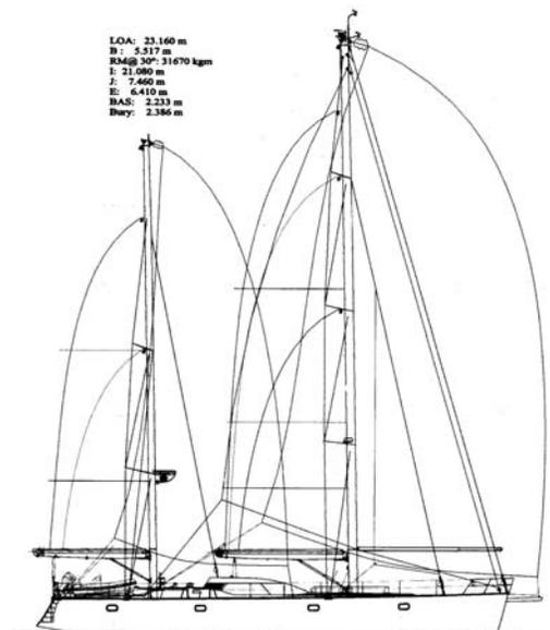
Figure 3 76' ketch without aft rigging (Tripp Design)
