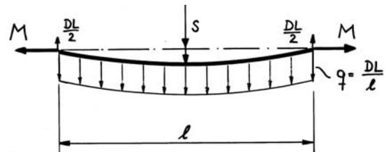
**Figure 8** Tension force in the leech or foot
