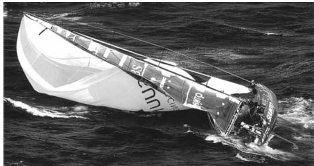
**Figure 1** Broaching of a Volvo Ocean Racer
