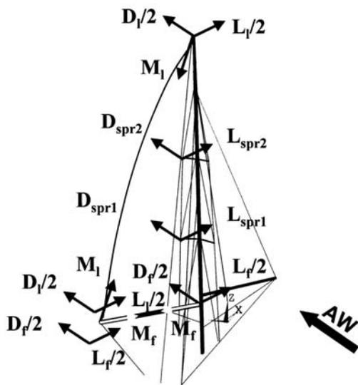
**Figure 6** All single forces of the load model for the main sail acting on the rig
