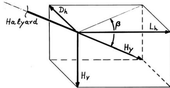
Figure 10 Forces at the spinnaker head
