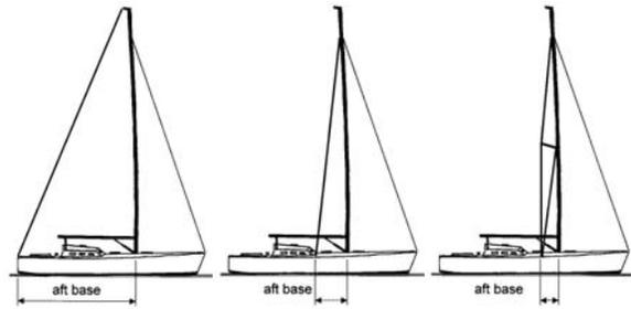
Figure 2 Aft staying bases depending on rig types
