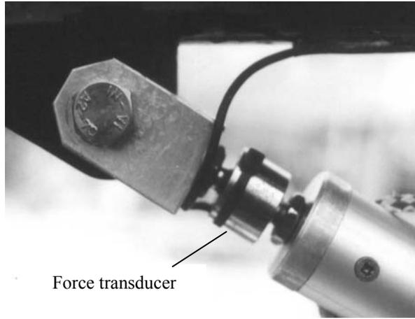
**Figure 13** Force transducer in the vang
