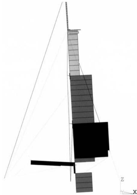
**Figure 16** Torque in the rig, AWA 135
