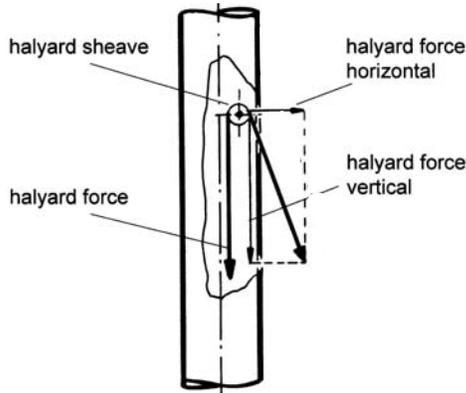
**Figure 11** Halyard forces applied at sheaves
