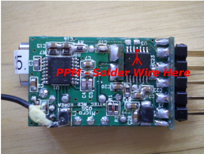
Fig. 4. Receiver PPM Bypass
